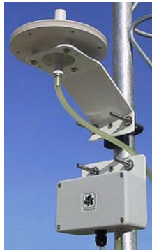
Barometer shown with 61002 Pressure Port
