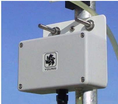
61202 Barometer mounted on mast.
