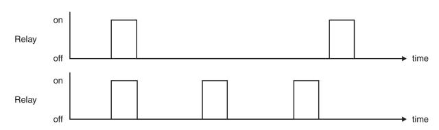
Frequency control - pulse frequency varies according to settings and control requirement
