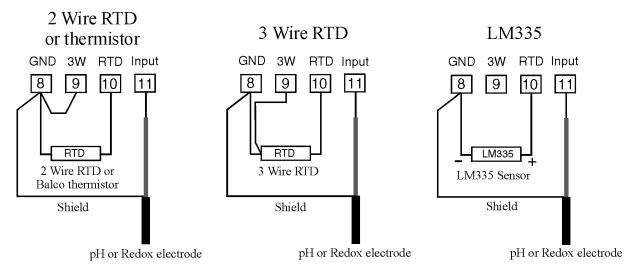
Termination of a typical pH electrode with temperature compensation
