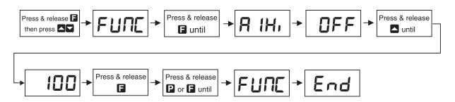
Example: Entering **CAL** mode to change decimal point function **dCPL** from **0** to **0.02**
