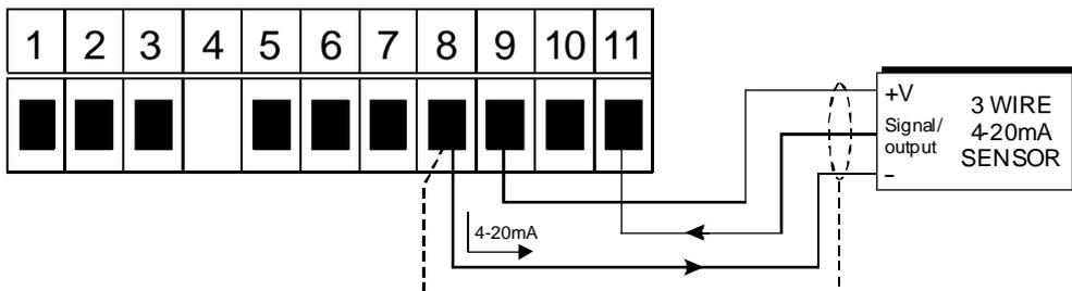
6. 4-20mA input - powered from optional  $\pm 12V$  (20mA) PM4 supply
