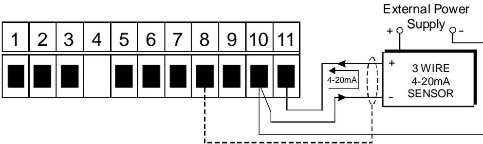
4. 4 wire 4-20mA input - externally powered sensor
