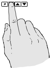
1. Remove power from the instrument. Hold in the **F** button and reapply power. The display will briefly indicate **CAL** as part of the "wake up messages" when the **CAL** message is seen you can release the button. Move to step 2 below.
