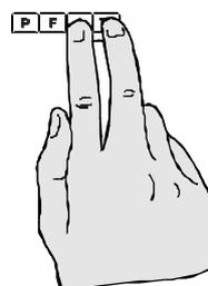
2. Within 2 seconds of releasing the **F** button press, then release the **▲** and **▼** buttons together. The display will now indicate **FUNC** followed by the first function.
