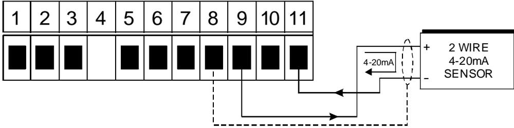
2. 2 wire 4-20mA input - externally powered sensor
