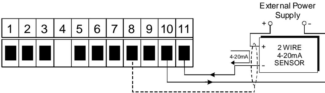
3. 3 wire 4-20mA input - externally powered sensor
