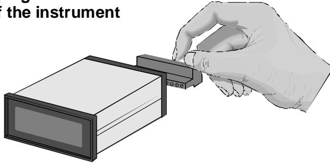
2. Remove 4 x self tapping screws from back cover, remove back cover by pulling it away from the instrument
