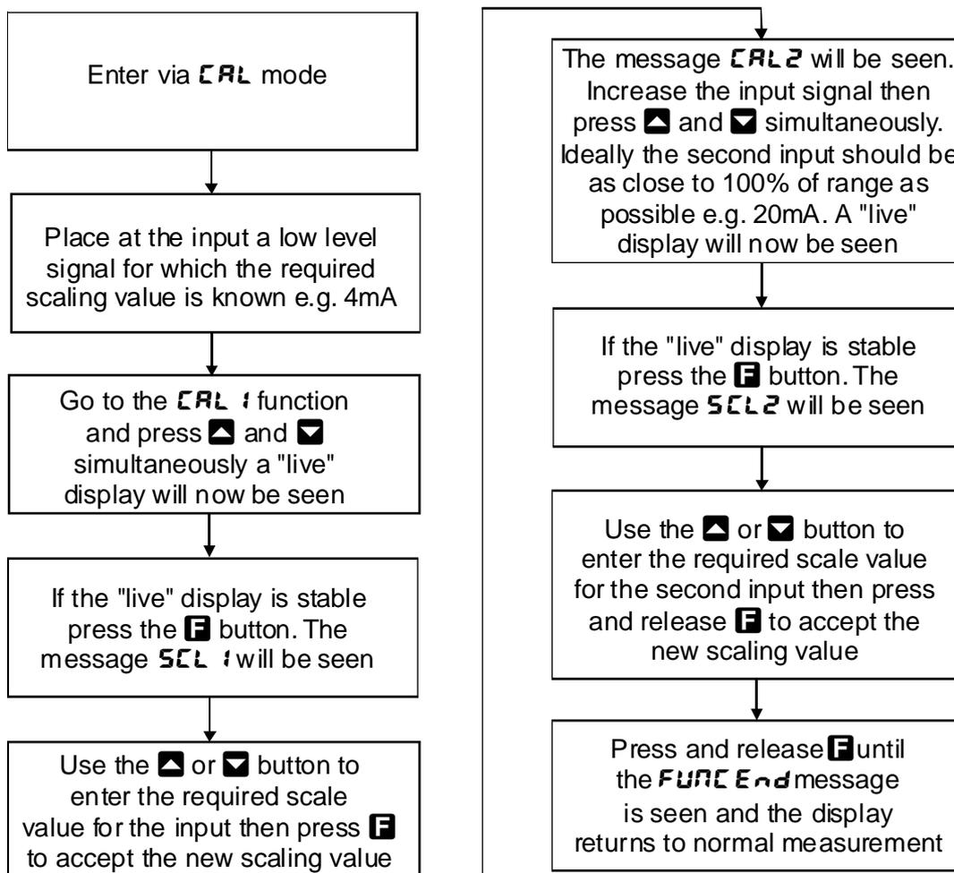
Note: If the "live" display at any scaling point is not stable then check the input signal for stability.
