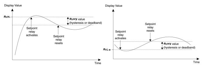
e.g. if **R** 1H is set to **50.0** and **R** 1HY is set to **3.0** then the setpoint output relay will activate once the display value goes above **50.0** and will reset when the display value goes below **47.0** (50.0 minus 3.0).
