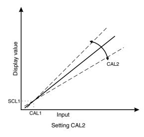
Example - Scaling using two live inputs
