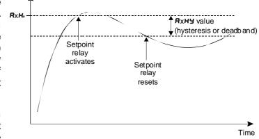
e.g. if **R IH**, is set to **50.0** and **R IHY** is set to **3.0** then the setpoint output relay will activate once the display value goes above **50.0** and will reset when the display value goes below **47.0** (50.0 minus 3.0).
