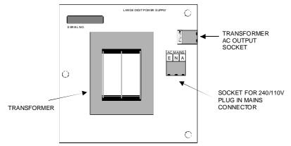
The transformer low voltage AC output goes to the power supply connector P1 on the main circuit board via the lead supplied.
