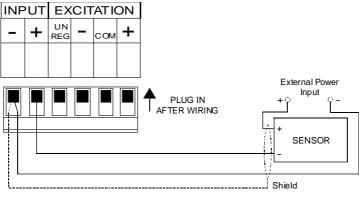
4. 2 wire 4-20mA input - powered from standard 18VDC supply (AC powered models only)
