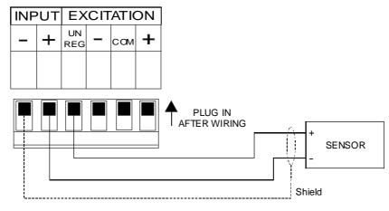
5. 3 wire ±20mA or 4-20mA input - powered from standard 18VDC supply (AC powered models only)
