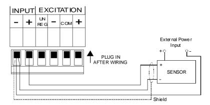
3. 2 wire ±20mA or 4-20mA input - externally powered sensor
