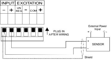
2. 3 wire ±20mA or 4-20mA input - externally powered sensor, common negative
