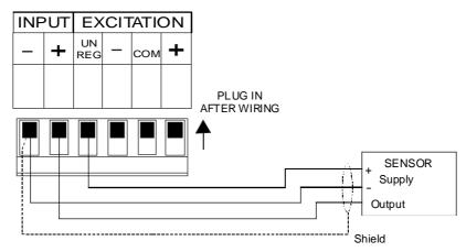
6. 2 wire ±20mA or 4-20mA input - powered from optional 24V (±12V) supply
