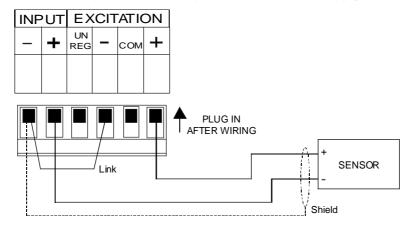
7. 3 wire ±20mA or 4-20mA input - powered from optional 24V (±12V) supply
