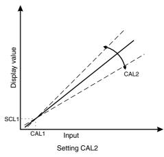
be seen instead of **SCL !** It is essential that the live input is different in value to the **CRL !** input e.g. for a 0-100V input use 100V as the **CRL2** live input. Note; it is not essential that exactly 0 and 100V are used as the live inputs for a 0-100V input scaling (or 0A and 5A) but the input values must be significantly different.
