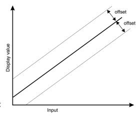
function. A "live" reading from the input will be seen, make a note of this reading. Press the button, the message **SCLE** will now be seen followed by the last scale value in memory. Use the or button to adjust the scale value to the required display value for that input. For example if the "live" input reading was **50** and the required display value for this input was **70** then adjust the **5CLE** value to **70**.
