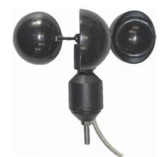
The model WS-MM-MW41 wind speed sensor uses the proven cup anemometer technology with a digital optical output for accuracy and durability. The anemometer has a photo-interrupter disc with 12 pulses per revolution to provide a high resolution frequency signal.
