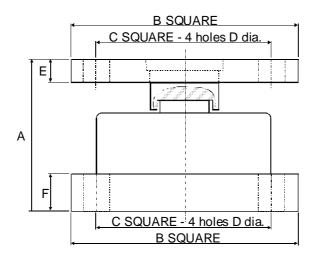
The complete mount is used with the **SG-LPX** in compression load applications.
